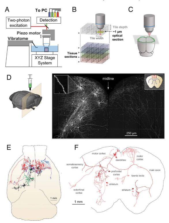
Fig. 4. The Janelia MouseLight Project to trace axonal projections of individual neurons. A) Schematic of the apparatus used for automated volumetric two-photon tomography. B) To image the whole mouse brain volume a collection of three-dimensional image stacks covering the full volume of the mouse brain are acquired serially. Tiles are overlapped in all three dimensions aid in image registration. C) The area of the brain for each section is imaged by first tracing the outline of the
